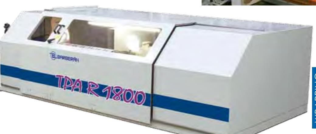
Automatic spool cutting machine by means of circular saw, with control board for the programming of the width and quantity of the cuts.
