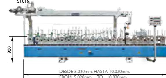
Machines for profile wrapping with wooden veneer, paper foils, low pressure laminates and similar materials.
